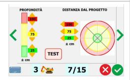
The LED panel setting mask is internal to the software and defines the precision ranges. It is also possible to combine sounds that always indicate the position of the bucket relative to the project.
